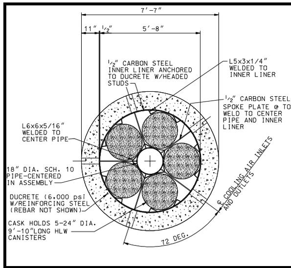
Figure 2. Cross Section of DUCRETE DWPF Cask
