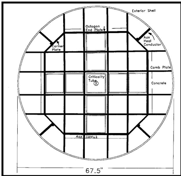
**Figure 4. CSI Cask Cross Section for 21 PWR Fuel Assemblies**
